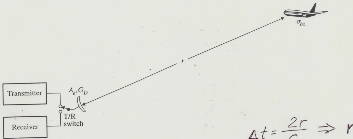
FIGURE 10-13 A monostatic radar system.
